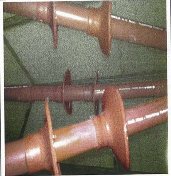
Photograph showing the sample with two "CABLINK" Heat Shrink Outdoor terminations after 1000 hours Salt-Fog test.
