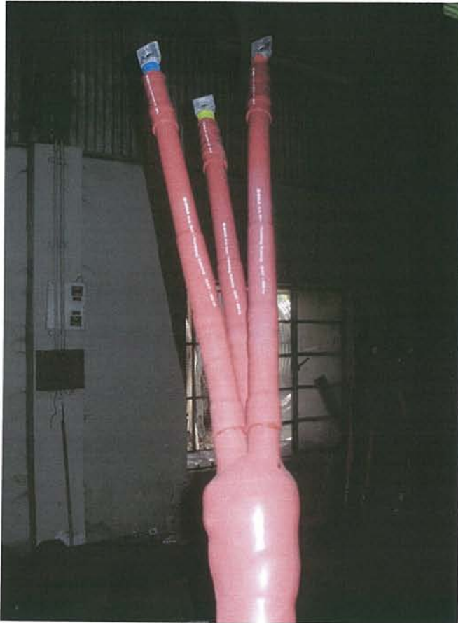
Photograph of Indoor terminations Before Humidity Test
