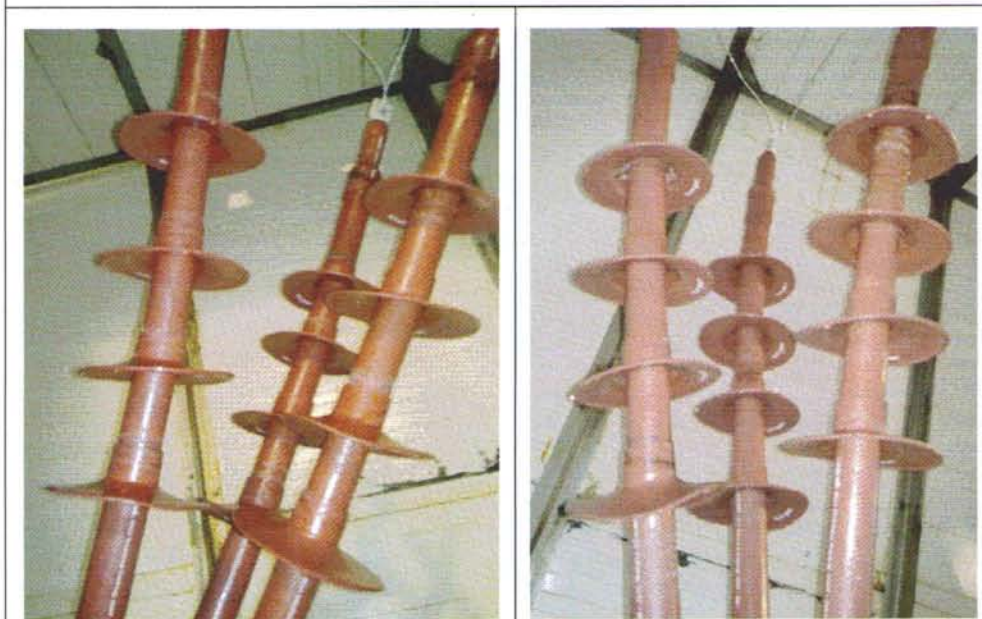
Photographs showing the sample Outdoor terminations After 1000 hours Salt-Fog test.
